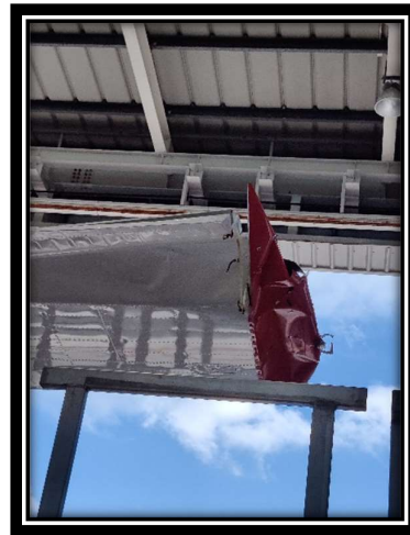
Fig 19: RH Wing tip - buckled
