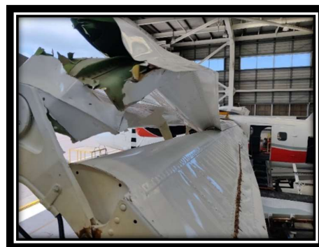
Fig 11: LH Outboard Fore flap
