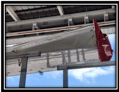
Fig 18: RH wing Aileron and trim tab – skin buckled RH wing tip
