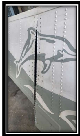
Fig 5: RH float outboard skin cracked at 7 th compartment line
