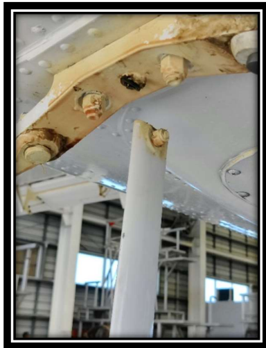
Fig 8: Vertical strut top eye bolt sheared
