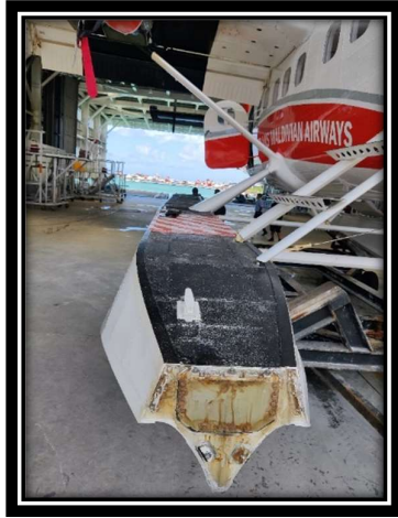
Fig 1: RH Float – Nose Bumper detached
