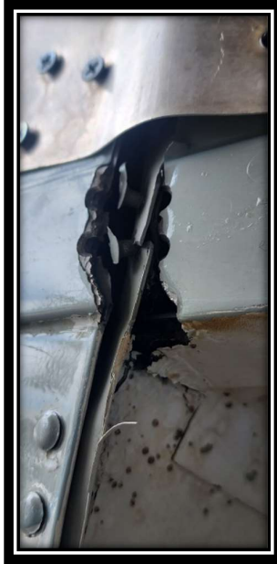
Fig 7: RH float inboard skin - ripped near compartment 6
