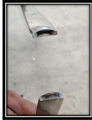
Fig 2: Float assembly flywire – snapped
