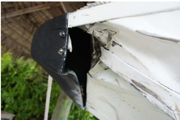
Image 5- LH Float damaged during the impact
