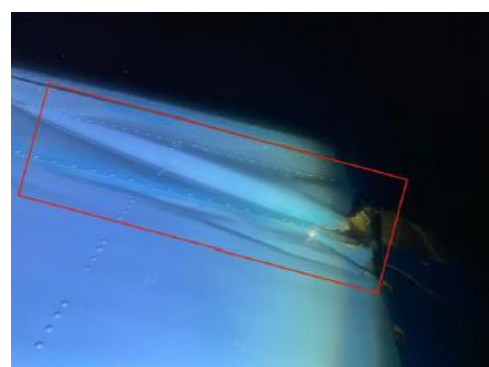
Figure 6: Left wing outboard training edge skin dented
