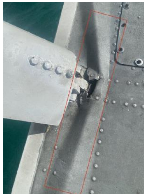
Figure 10: Left float top skin has been dented and damaged at number 6 bulkhead
