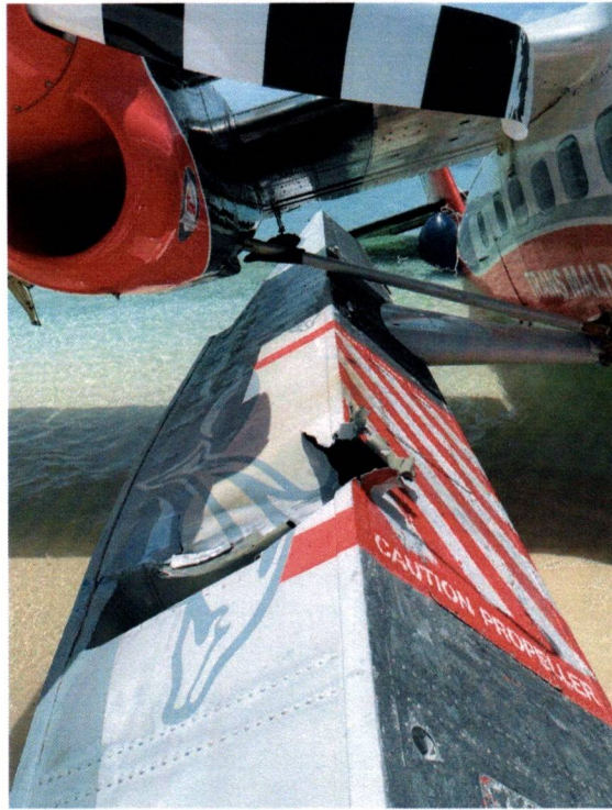
Fig 9: Damages on RH float
