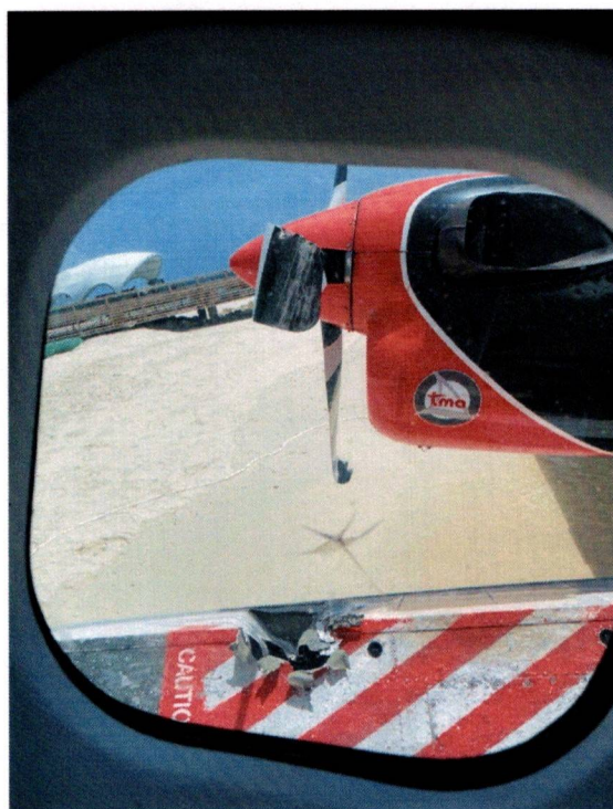
Fig 8: Damages on RH propeller and RH float
