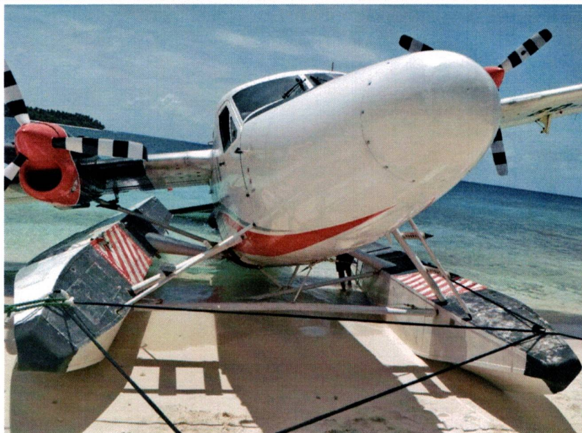
Fig 3: Aircraft beached – RH float detached at aft fitting
