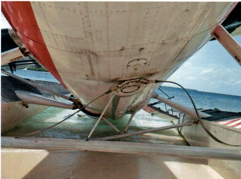
Fig 2: Flywire RH snapped; LH buckled
