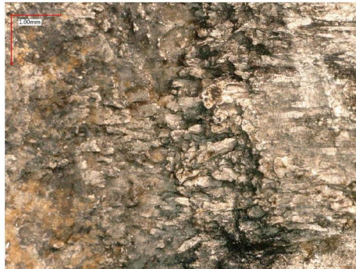
Fig. 6 A higher magnification image of the fracture surface reveals corrosion deposits and intergranular cracking corresponding to the highlighted area from Figure 5.
