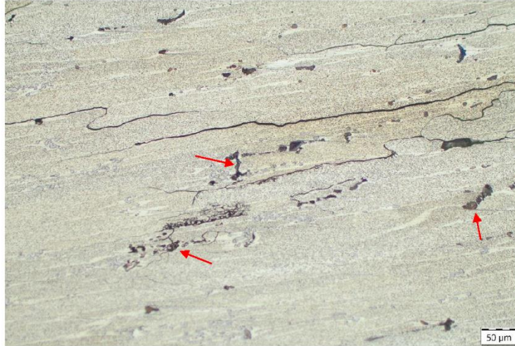
Fig. 15 The highlighted area from Figure 14 is shown at higher magnification. The surface exhibits intergranular cracks and the formation of precipitates along grain boundaries. Corrosion attack is evident around the precipitates, as indicated by the red arrows. Keller's reagent.
