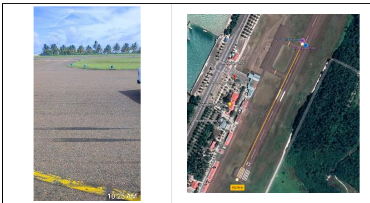
Figure. 10: Tyre markings showing touchdown point plus remaining Runway length
