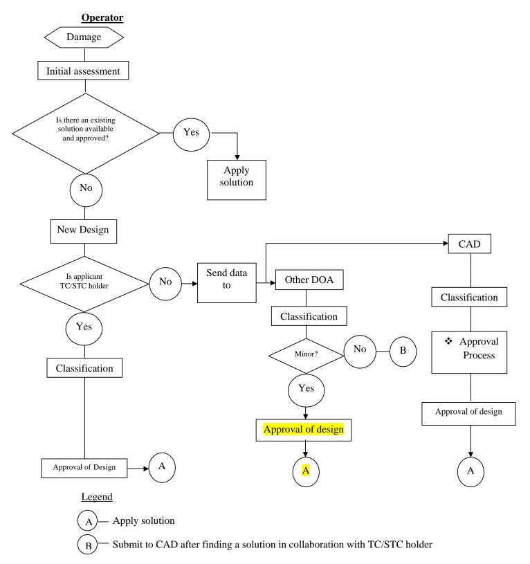
❖ In case of major repair CAD would require design solution/data from TC/STC holder
