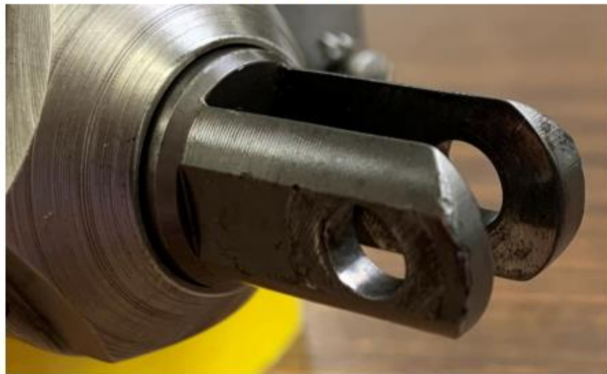
Figure 2 Beta Valve Clevis Damage
