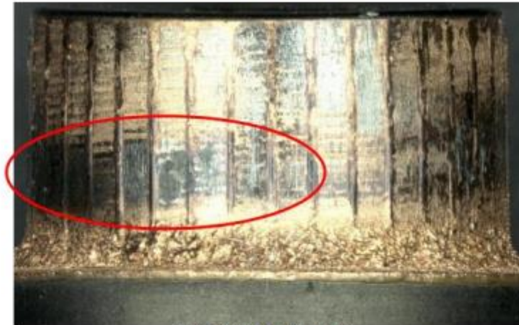
Figure 4 Braze Joint Porosity
