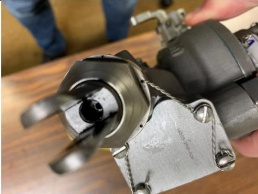
Figure 1 Separated Beta Valve Assembly
