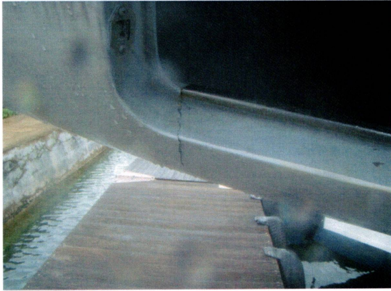
Fig 5: Nose skin cracked STA 100
