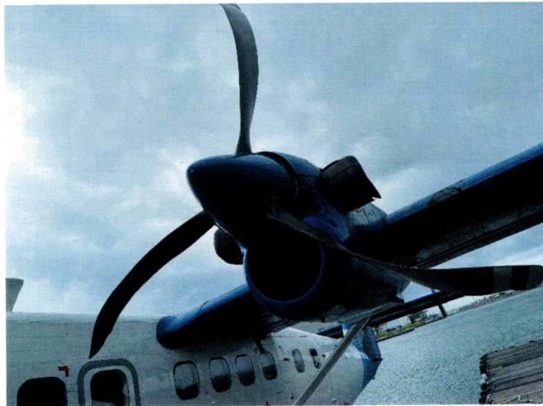
Fig 6: LH Propeller damaged
