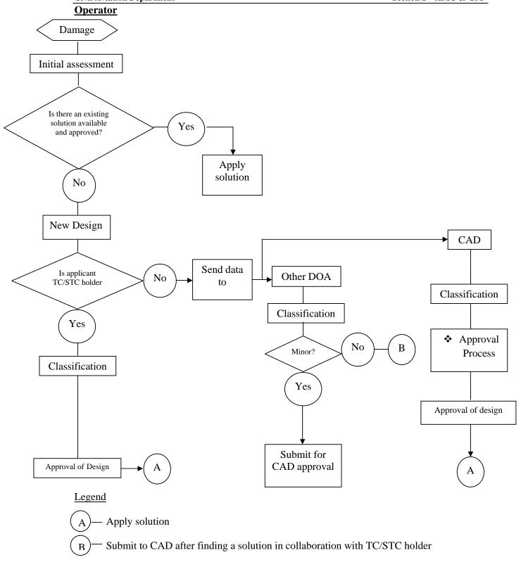
❖ In case of major repair CAD would require design solution/data from TC/STC holder
