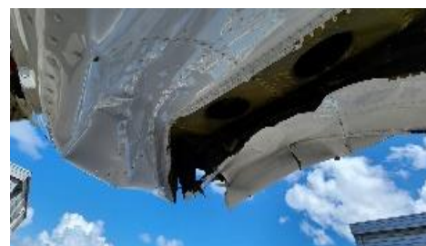
Figure 10 LH Wing Leading Edge Damage
