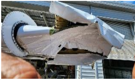
Figure 12 LH Wing Leading Edge Damage
