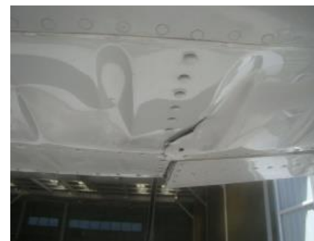
Figure 9 LH Aileron Damage
